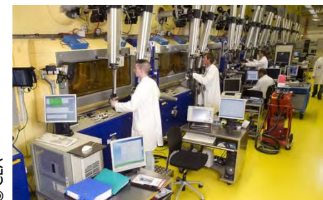
Line M constituted with 19 hot cells for surface characterization.
