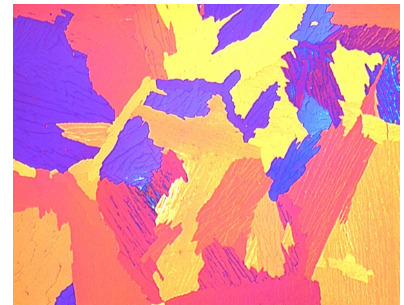
Polarized light optical microscopy of the prior- \beta structure (CEA/DMN/SRMA)
